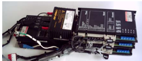
Figure 4. Detail of the power drivers included in the power module.
